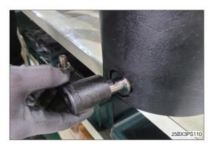
(18) Assemble snap ring on parking lever pushing (18). Mark a point for checking for proper assembling.
