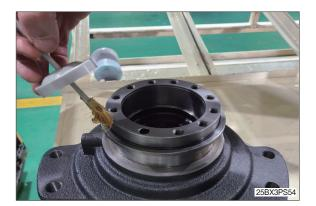
(3) Assemble differential gear case (11) on LH axle housing (2).
