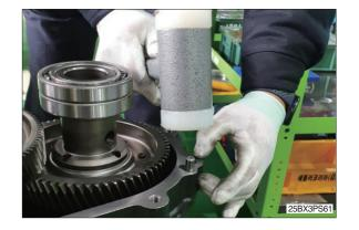
(7) Mark points on LH axle housing and the heads of socket-head bolts for checking for proper assembling.
