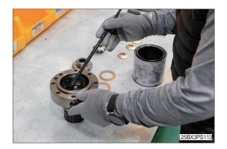
(2) Lubricate gear, washer and shaft with grease.
