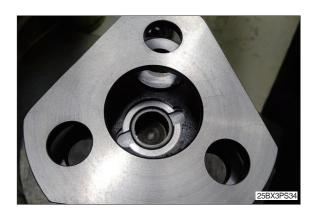
(2) Assemble thrust washer and needle valve bearing (7, 8) on grease-lubricated carrier shaft.
