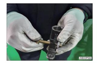
(9) Assemble key (2) on parking lever pushing (6).
