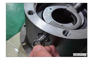
(13)Lubricate the surface of O-ring with grease.
