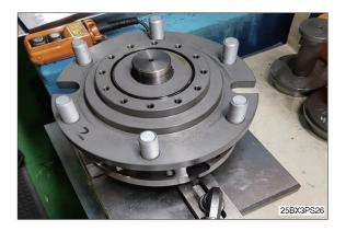
(11) Assemble lock plate on carrier shaft, and then fasten lock nut lubricated with Loctite 277 on carrier shaft.
