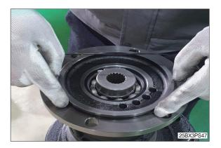
(7) Assemble dowel pin (6) on brake housing (7).
