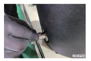
(10) Assemble parking lever pulling assembly on parking lever pulling (6).
