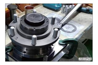
(15) Fasten socket-head bolt (1) lubricated with Loctite 277 on wheel cap (2).  $\cdot$  Fastening torque : 3.3 $\pm$ 0.2 kgf  $\cdot$  m
