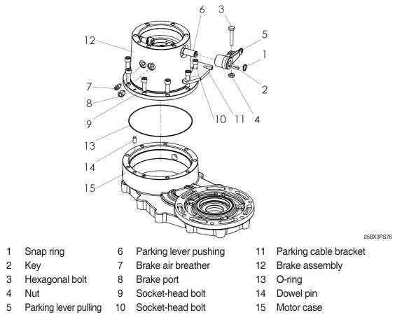
(1) Once snap ring (1) is removed, remove parking lever pulling (5) from parking lever pushing (6).
