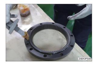
(4) Assemble ring gear assembly on axle housing (6).
