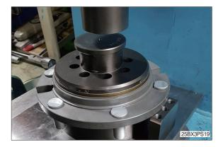
(4) Lubricate ring surface inside adaptor(6) with proper amount of grease.
