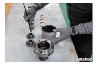
(3) Assemble pinion gear, shaft and washer on differential gear case (7) and differential cover gear (9).
