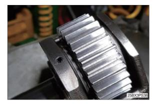
(6) Caulk with a tool to prevent spring pin from removal from carrier shaft.
