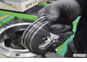
(5) Fasten hexagonal bolts (6) on brake piston (9).
