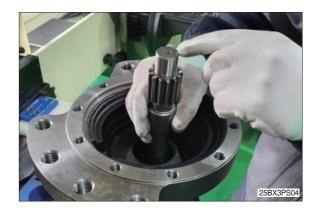
(2) Care shall be exercise to protect O-ring(4) from damage when assembling it on ring gear (5).
