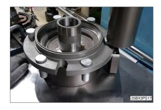
(2) Apply ThreeBond on the outer surface of oil seal (8).
