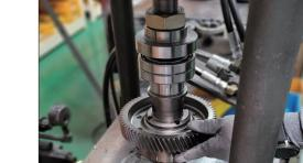
(9) Assemble ball bearing (4) and brake hub (3) on differential case assembly.
