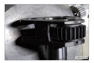
(4) Assemble planetary gear shaft (3) on carrier shaft (1) by aligning with hole of the latter.
