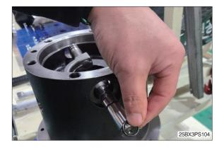
(16)Lubricate the surface of O-ring with grease.
