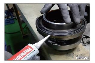
(3) Make use of jig and press to assemble oil seal (8) on adaptor (6).
