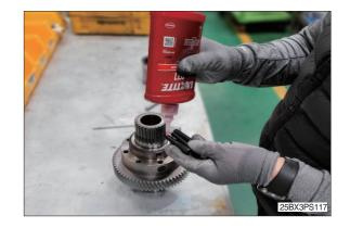
(6) Assemble 8 socket-head bolts (6) on differential gear case (7).
