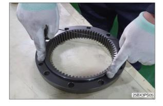
(3) Lubricate the surface of O-ring with grease.
