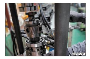
(10) Assemble snap ring (2), and then mark a point for checking proper assembling.
