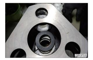
(3) Assemble 3 planetary gear assemblies on carrier shaft (1).
