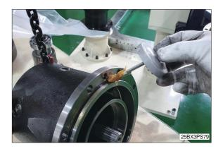
(4) Mount brake assembly on motor case (15).
