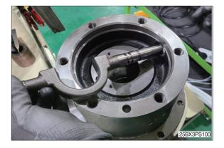
(12) Assemble 2 O-rings on parking lever pushing (18).
