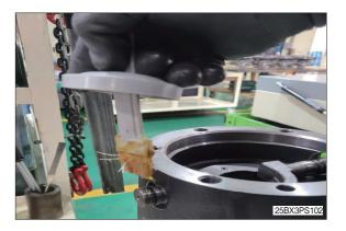
(14) Assemble snap ring (14) on parking lever pushing (18). Mark a point for checking for proper assembling.
