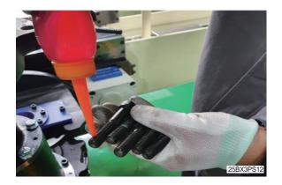
(10) Assemble socket-head bolt (1) on axle housing (6).
