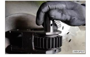
(5) Assemble 3 spring pins (2) on carrier shaft (1).
