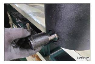
(11)Assemble snap ring (1) on parking lever pushing (6). Mark a point for checking proper assembling.
