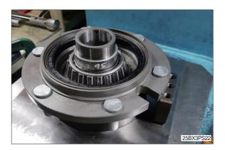
(7) Make use of jig and press to assemble final housing (11) and taper roller bearing (12) on adaptor (6).
