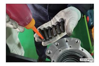
(13) Fasten 11 socket-head bolts.  $\cdot$  Fastening torque : 9  $\pm$  0.5 kgf  $\cdot$  m
