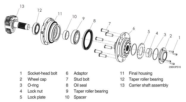
(1) Remove socket-head bolt (1) from wheel cap (2).
