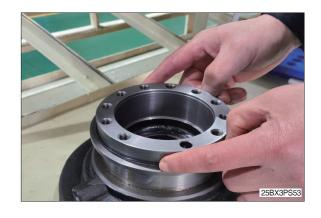
(2) Never forget to lubricate the surface of O-ring (12) with grease.
