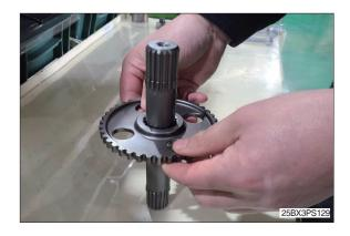
(2) Assemble snap ring (1) on center shaft(3).
